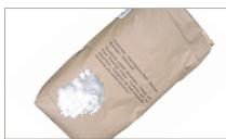
TwinLite - Diatomaceous Earth used as filter aid for water treatment and completion fluids.
